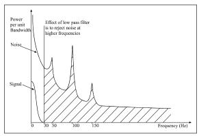
Figure 5: Effect of Low Pass Filter
