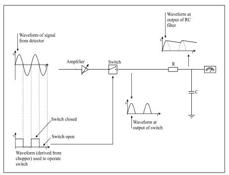
Figure 8: Synchronous Filter
