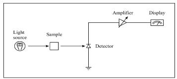
Figure 3: Schematic of Lock-in Device
