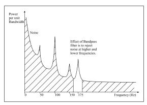
Figure 6: Effect of Bandpass Filter at 175 Hz
