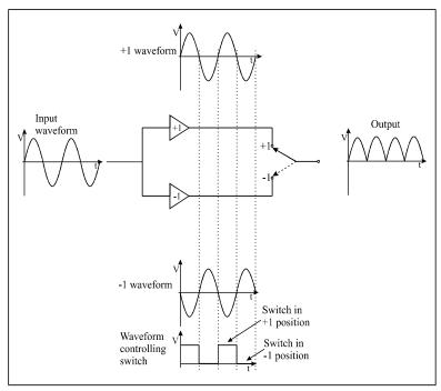
Figure 10: Rectifier operation
