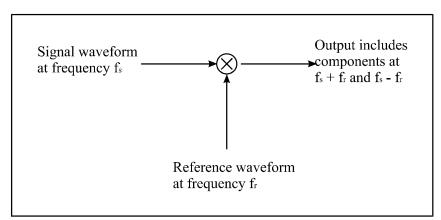
Figure 9: Alternative visualisation of phase detector
