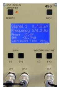
Figure 1: Front panel of 496 lock-in amplifier/ADC
