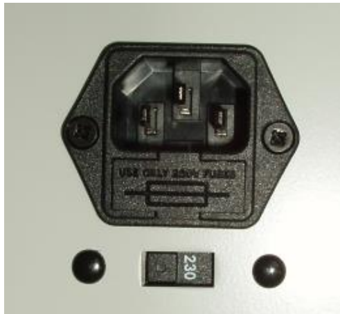
Figure 2.4: Voltage selector displaying voltage in use
