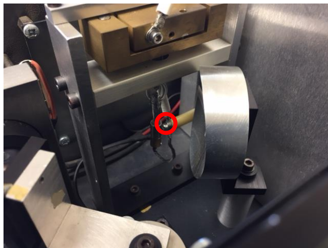
A5.2: Remove this screw to remove the cable connecting the xenon lamp
