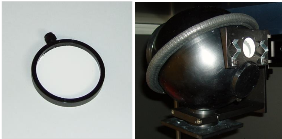
Figures 6.7 & 6.8: Specular “includer”, and fitted to DTR6
