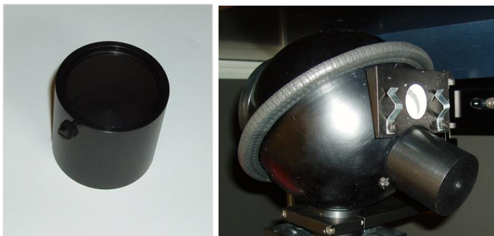
Figures 6.5 & 6.6: Specular trap, and fitted to DTR6
