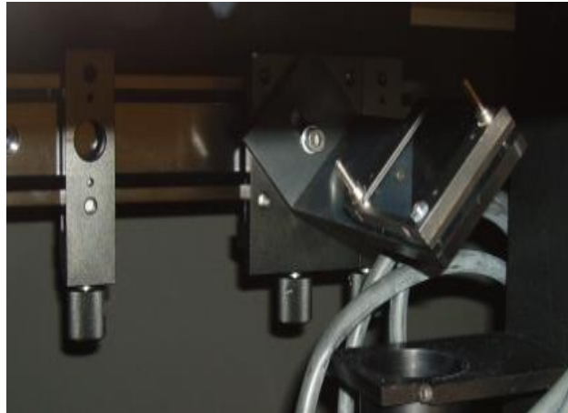
Figure 6.3: Relay mirror reflecting light toward DTR6
