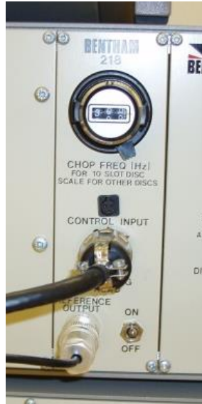
Figure 9.2: On/Off switch to use or arrest the chopper
