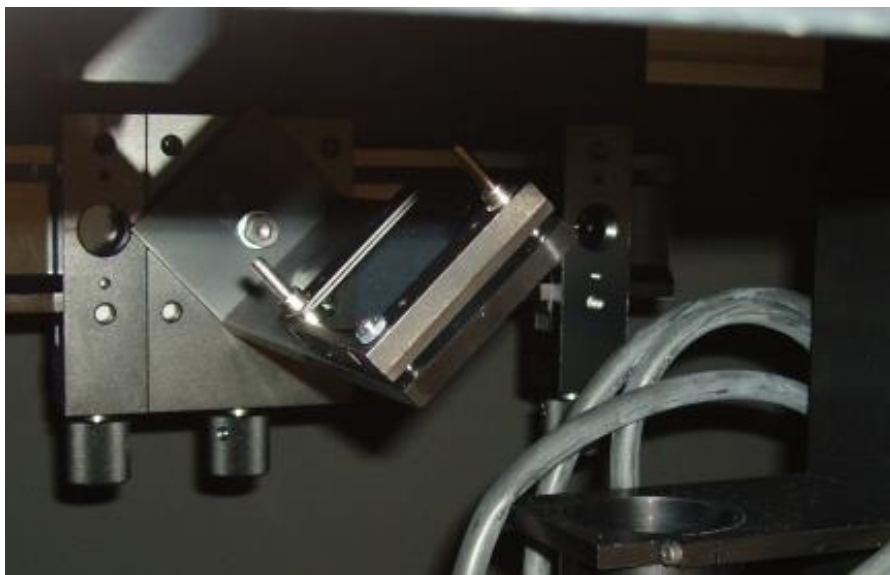
Figure 8.1: Relay mirror out of beam (EQE)
