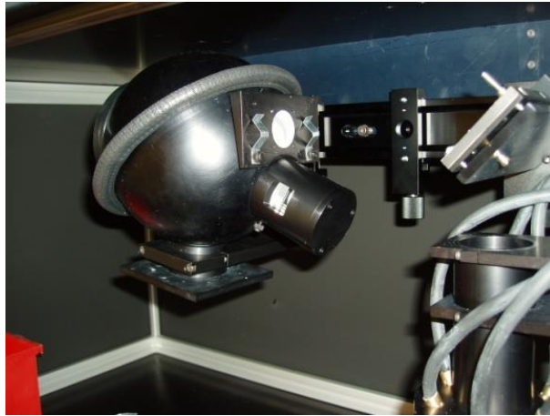
Figures 6.13: Sample port viewer installed
