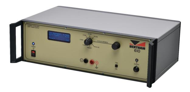
The Bentham 610 is a constant current power supply designed for use with stabilised light sources and calibration standard sources. The unit is capable of sourcing 10.4 A DC current at a voltage of up to 26 V.
