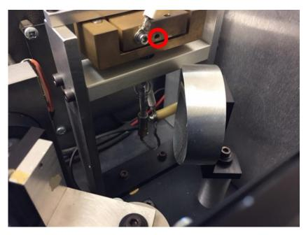
Figure 6: Grub screw that releases the top of the xenon lamp
