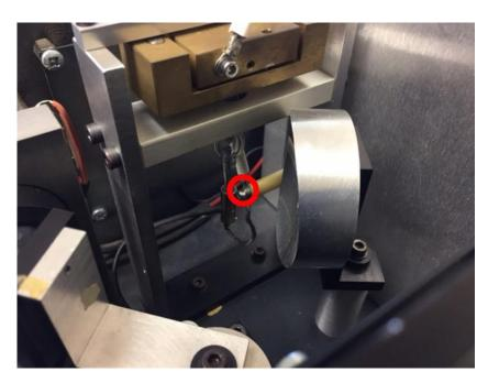
Figure 7: Remove this screw to remove the cable connecting the xenon lamp
