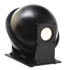
The LumiCal50 comrpises a barium sulphate coated integrating sphere with 100W halogen lamp to ensure uniform high luminance over the exit port. Attached to the left hand wall of the LuxCal250, the output of the LumiCal50 is brought to 2856K by using varying current and colour shift filters, whilst various luminance levels are obtained using ND filters.
