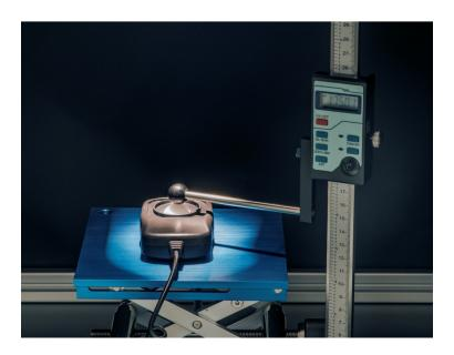
A laser alignment aid is swung into the beam to ensure centralisation of the DUT
