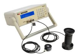
The ORM400 picoammeter, associated with a reference lux and luminance meter with UKAS accredited calibration, is used to determine the reference lux or luminance level of the LuxCal250/ LumiCal50.
