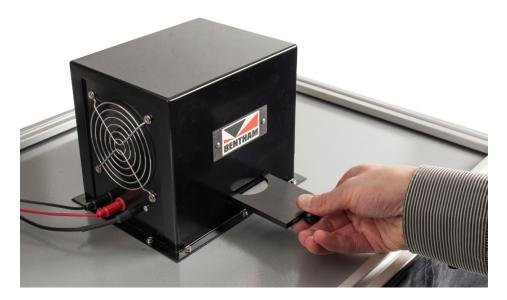
The sample plane of the LuxCal250 is located 175mm above the base of the unit. A height gauge is provided to ensure that the device under test is placed at this position; a lab-jack is used to accommodate the height of the device under test.
