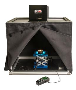
The LuxCal250 houses a halogen source to the top which is set to 2856K by use of varying lamp current and installing a colour shift filter on the table to the top of the chamber. Various levels of illuminance are obtained by use of ND filters installed in the lamp housing from outside the chamber. The calibration certificate tells the user which filters to use.
