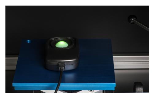
With the DUT set up, a curtain allows ensuring the device illuminated solely by the calibration source, whilst giving access to the meter to read results.
