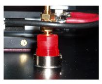
Adjust lateral position by turning brass screw accessed through port to side of, housing, found behind a plastic cover
