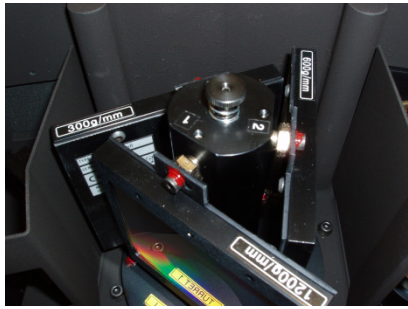
Figure 8:- Long pin screwed by hand until finger-tight
