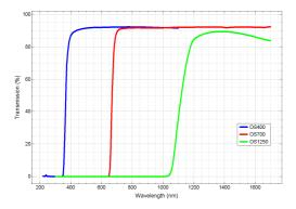
Figure 2:-Typical OS filter transmission
