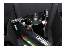
Figure 8:- Long pin screwed by hand until finger tight
