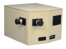
Figure 1:- TMS300 monochromator
