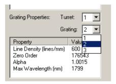
The zord and alpha parameters for each grating are obtained from the calibration certificate.
