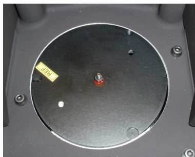
Figure 7:- Turret base showing reference pin and screw attachment
