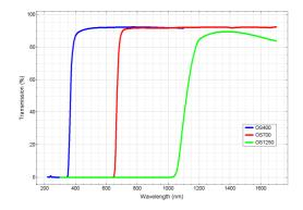
Figure 2:-Typical OS filter transmission
