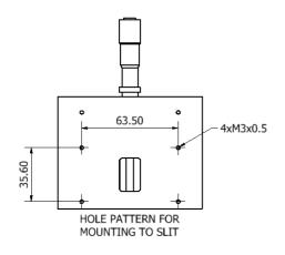
Figure 3: TMc150 slit hole pattern
