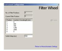
The insertion wavelength relevant to the filter in a given position should be input. The order need not be ascending.
