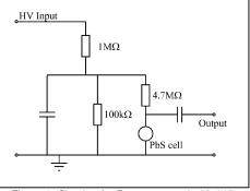
Figure 1: Circuitry for Detectors used with 215
