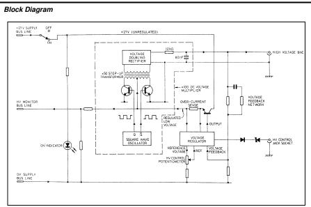
Figure 2: High Voltage Supply Schematic
