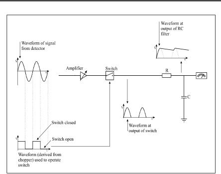
Figure 6: Synchronous Filter
