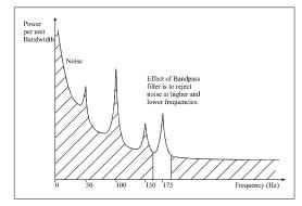
Fig 4 Effect of Bandpass Filter at 175 Hz.
