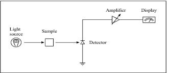
Figure 1: Schematic of Lock-in Device
