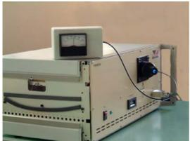
Figure 6:- Optical output measurement during alignment
