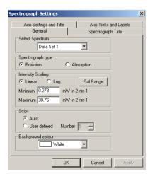
General: Define spectrum as being emission or absorption type, apply linear/ logarithmic scale, define scale, range, and number of bars in spectrograph. Axis settings & title: Define axis and fonts
