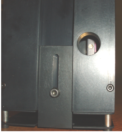
Figure 6: Load bearing feet dropped and locked in place by tightening screw
