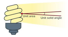
The radiance of a source is defined as the power emitted per unit area of the luminous surface into unit solid angle. The product of area and solid angle is called the geometric extent, which is at best conserved in any optical system. Radiance can be decreased by filters or diffusers, but not increased by any optical system. It is for this reason that radiance is used to account for light perceived by the eye through its photometric equivalent, luminance.
