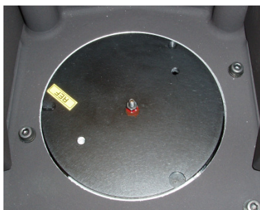
Figure 3:- Turret base showing reference pin and screw attachment
