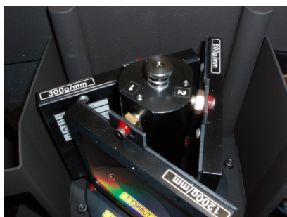
Figure 4:- Long pin screwed by hand until finger tight
