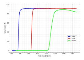
Figure 2:-Typical OS filter transmission
